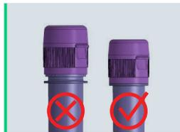
Make sure each test tube is fully locked
