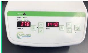
Set the temperature to 37°C and press <on>
