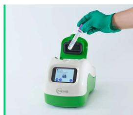
Place the test tube into the luminometer
