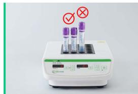
Fully insert the test tubes inside the wells of the incubator
