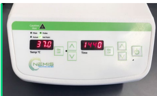
Set the temperature to 37°C and press <on>. Set the timer to 1440 minutes [24h].
