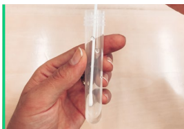
Open the test tube and swirl the swab inside the enrichment broth for min. 5s. Discard the swab.
